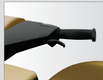
iBR™ (Intelligent Brake & Reverse) brake lever
